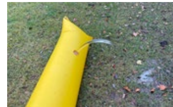
After the drainage cap is removed water will drain out of the tube.
