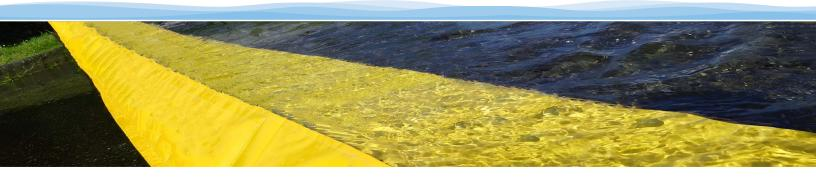
The Stingray™ Self-Deploying Water Dam is a flexible yet effective flood control dam system used to stop and hold back water. As water accumulates inside the dam pocket chambers, it ballasts the bottom of the fabric; combined with the traction strips on the underside, the water dam stays in place. As water enters the barrier's "pocket", water pressure builds up and this causes the barrier to open up in a V-shape.
