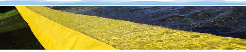
The Stingray<sup>™</sup> Self-Deploying Water Dam is a flexible yet effective flood control dam system used to stop and hold back water. As water accumulates inside the dam pocket chambers, it ballasts the bottom of the fabric; combined with the traction strips on the underside, the water dam stays in place. As water enters the barrier's "pocket", water pressure builds up and this causes the barrier to open up in a V-shape.
